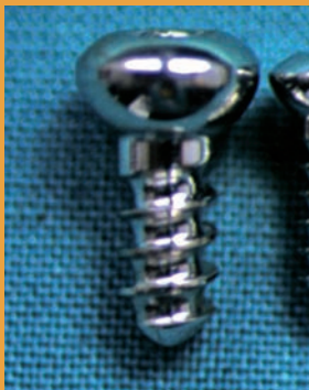
FIGURE 119. Image of a screw. Note the conical form of the "head", which is similar to the body of a spinning top.
