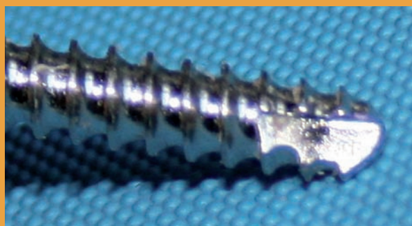
FIGURE 103. Detailed image of the tip of a self-tapping screw. Note its similarity with the tip of a thread insert.
