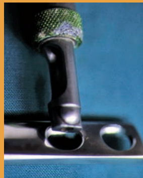
FIGURE 120. End of the guide designed to fit into the holes of DCP plates.
